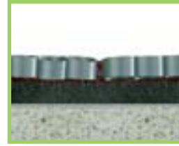
Fig. 2 • Standard grid surface subject to +100° temperature
